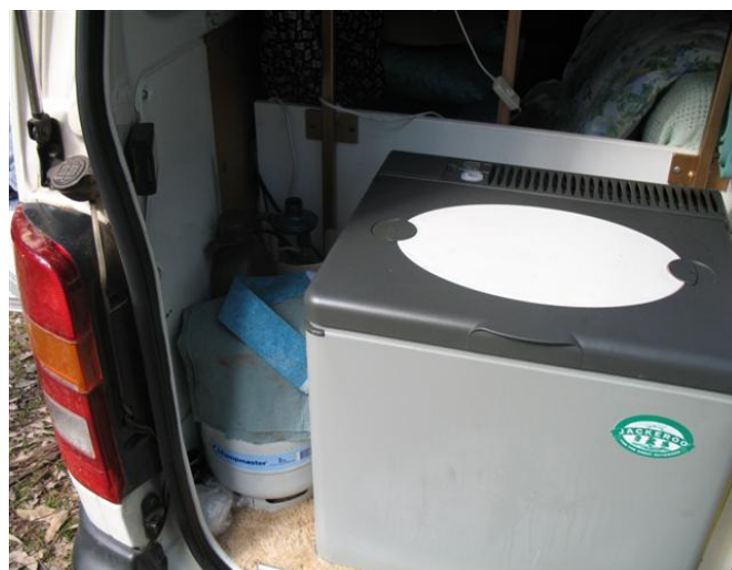
Location of refrigerator inside the unventilated campervan - note the gas cylinder beside the appliance.
